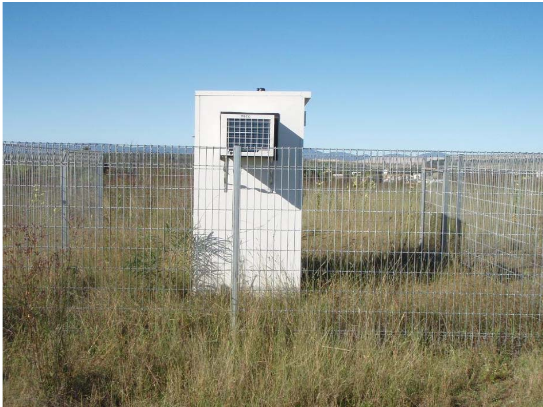
Figure 13: Example of a TEOM in the field
