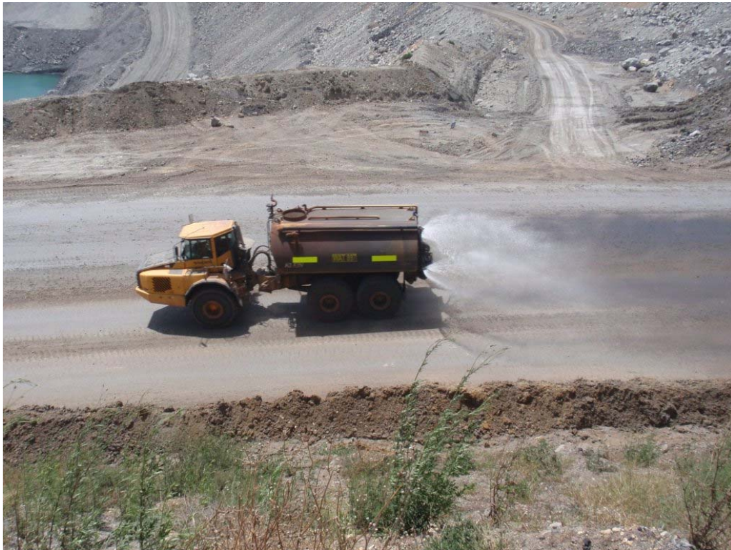
Figure 6: 30,000L Volvo Wobbly Water cart in operations at Werris Creek
