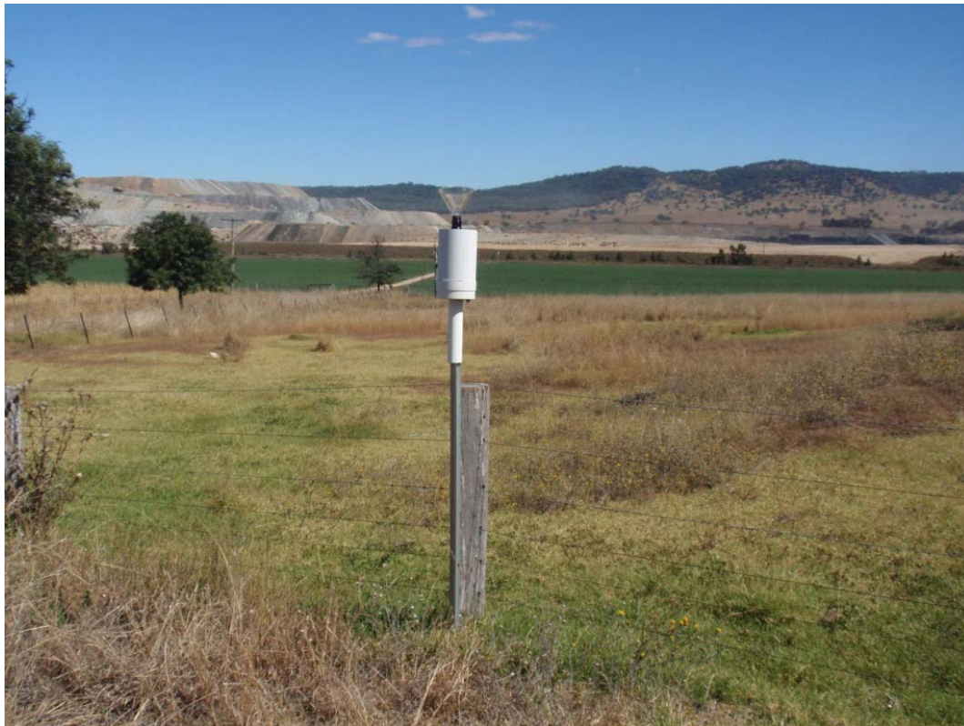
Figure 10: Example of Dust Deposition Gauge
